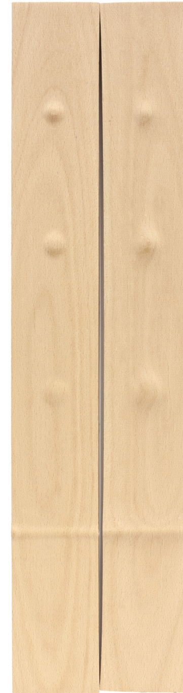
Fig.36. Beech samples after planing and steaming
