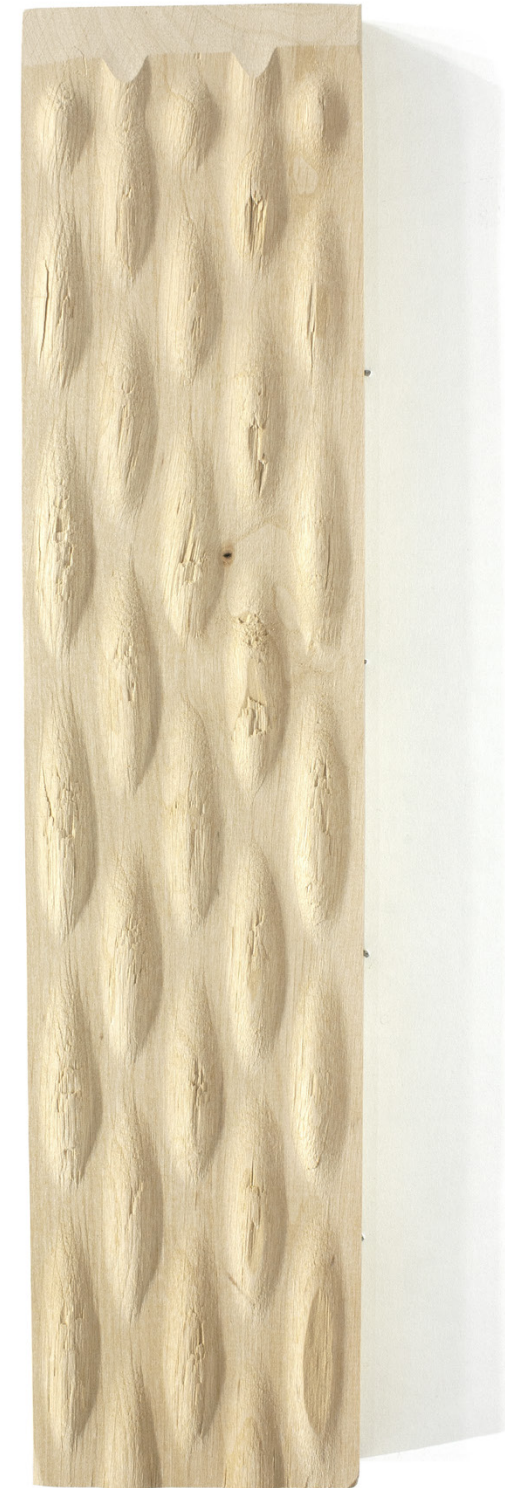
Fig.62. Embossed pattern made with 3D-printed pressing tool
