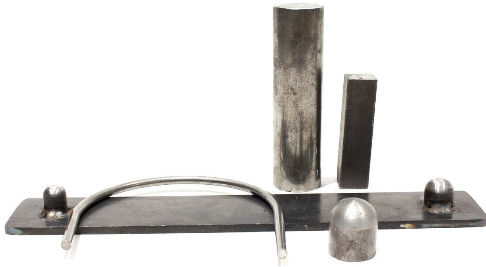
Fig.58. Metal profiles used to test different shapes for the embossments
