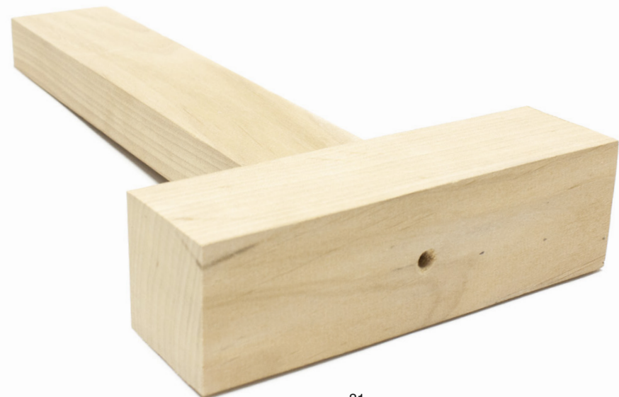
4. The joint is assembled whereafter steam is injected in to the joint through a hole. The indented fibers on the tenon retain their original shape and lock the two pieces together.
