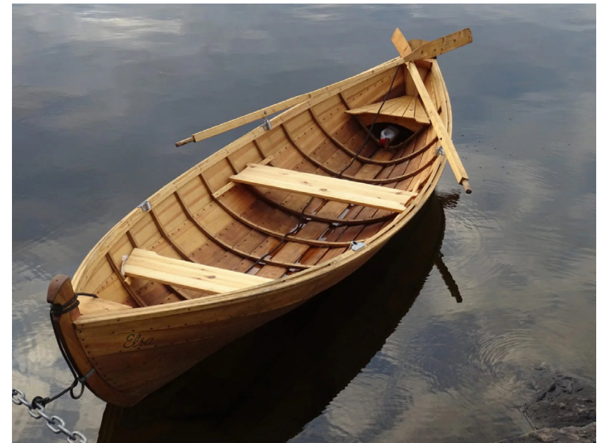
Fig.42. Wooden boats are made watertight by letting the seams swell together in water.
