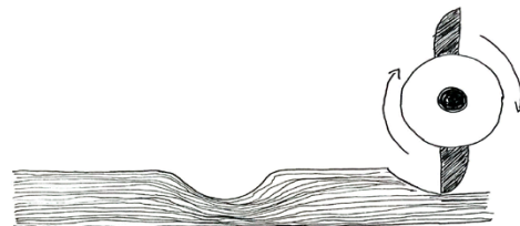
2. The surface is planed until the indent disappears.
