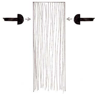
1. Indents are pressed on both sides of the tenon blank.
