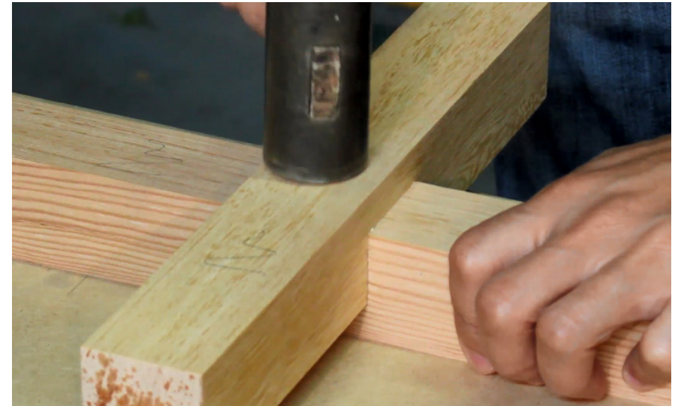
Fig.44. Kigoroshi used in a halving joint
