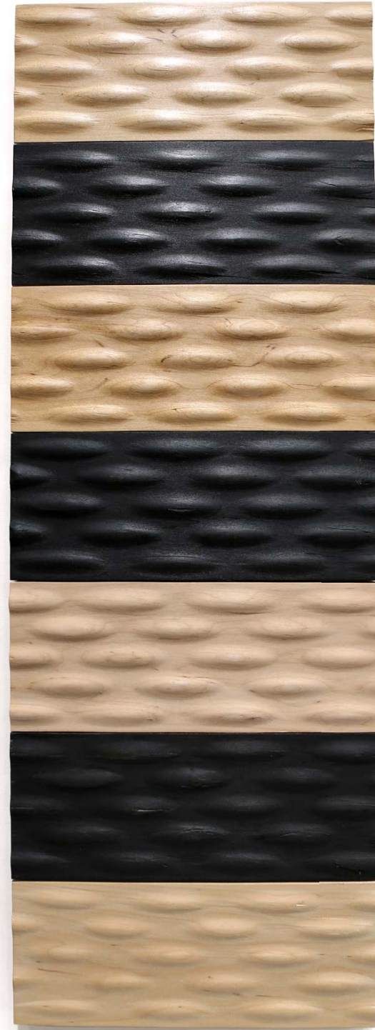
Fig.73. Surface treatment tests. From top down: 1. Danish oil, 2. Ink + Danish oil, 3. Osmocolor 3032, 4. Ink + Osmocolor 3032, 5. Osmocolor 3041 Valkotammi, 6. Ink + Soap, 7. Soap.
