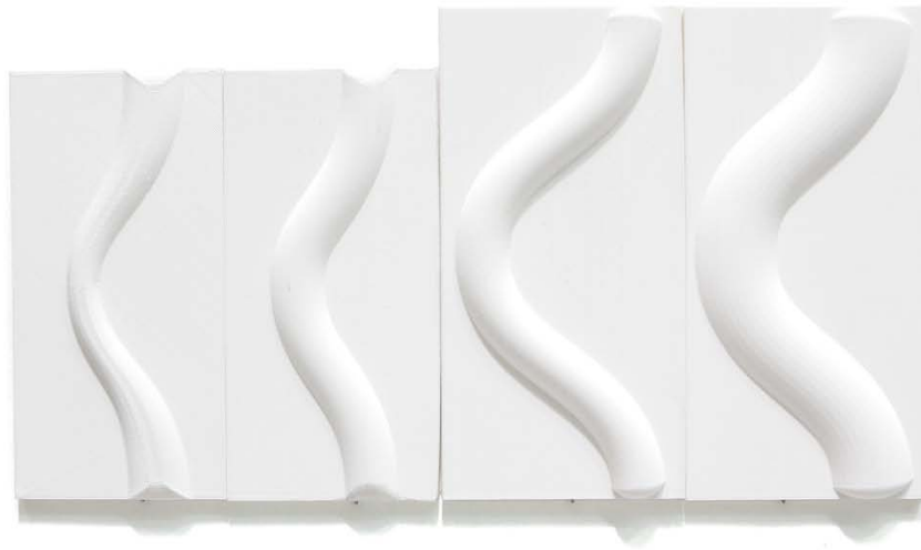
Fig.71. 3D-printed pressing tools with wave pattern
