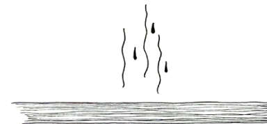
3. Moisture and heat is applied on the indented area.
