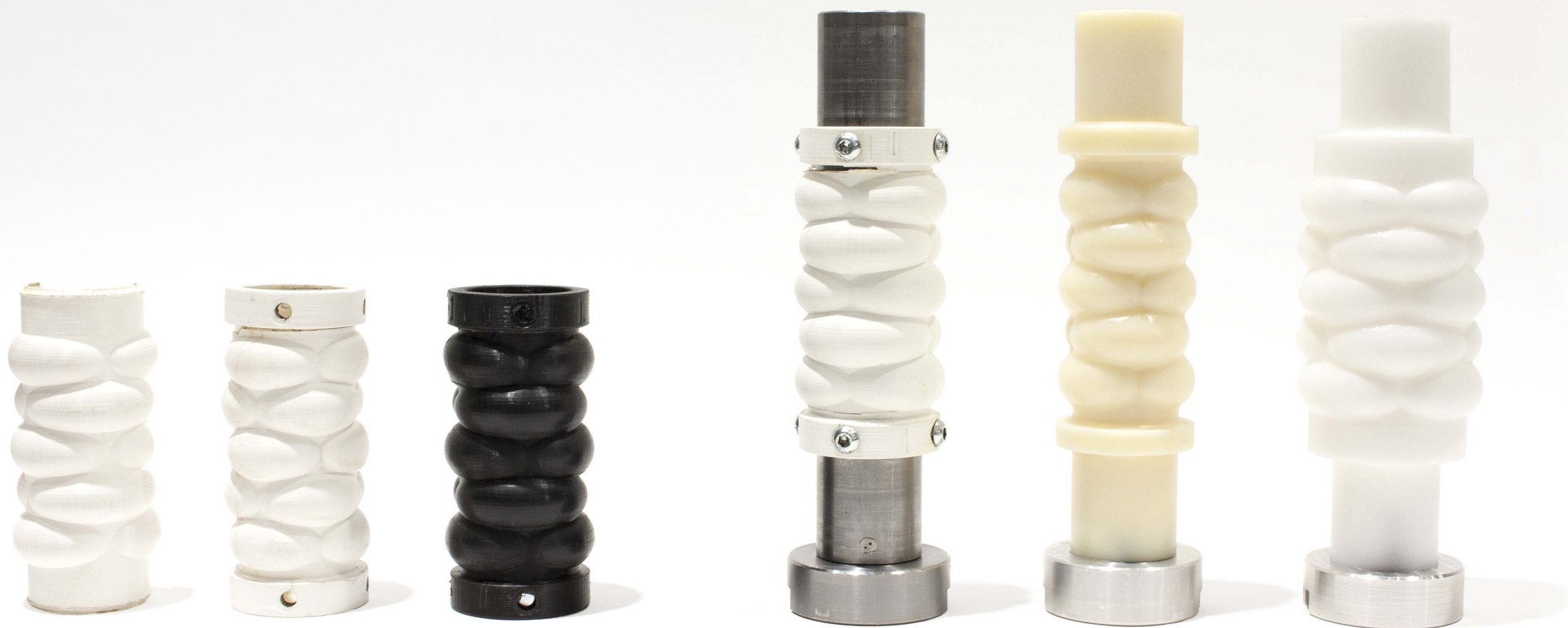
Fig.65. The development of the patterned pressing tool for the cylindircal press. From left to right, 1.-4. 3D-printed PLA, 5. CNC-milled nylon(PA), 6. CNC-milled POM.
