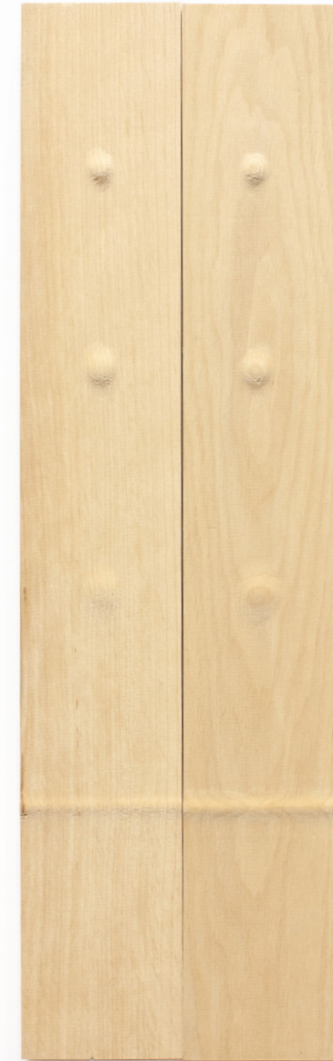
Fig.33. Alder samples after planing and steaming
